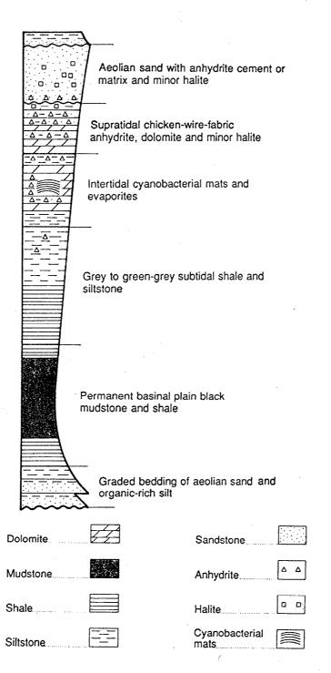
Figure 13. Idealised complete cycle of the coastal sabkha deposits of the upper Alinya Formation in Giles 1 well
