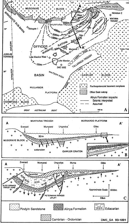
Figure 17. Idealised sedimentary basin and distribution of the Alinya Formation in the Munyarai Trough and Murnaroo Platform
