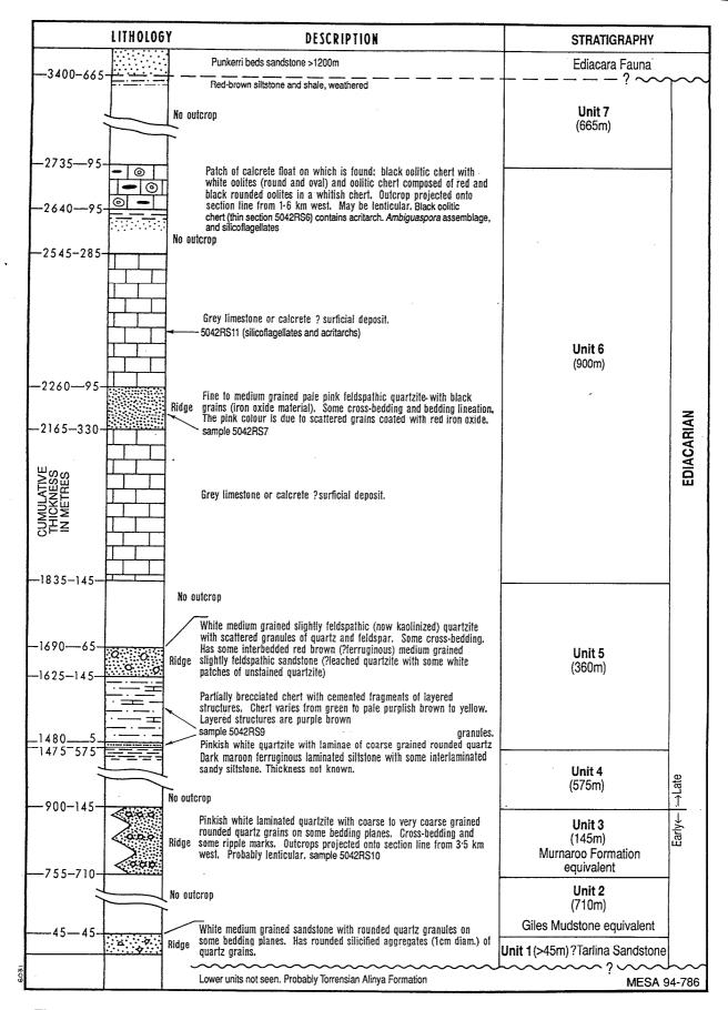
Figure 6 Type section of the Wright Hill beds
