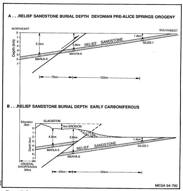
Figure 18 Suggested pre-orogenic (A) and post-orogenic (B) depths of burial for the Relief Sandstone
