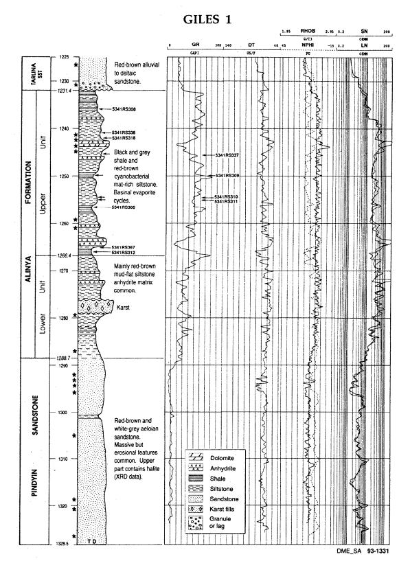
Figure 8. Detailed lithological description of the Pindyin Sandstone and Alinya Formation
